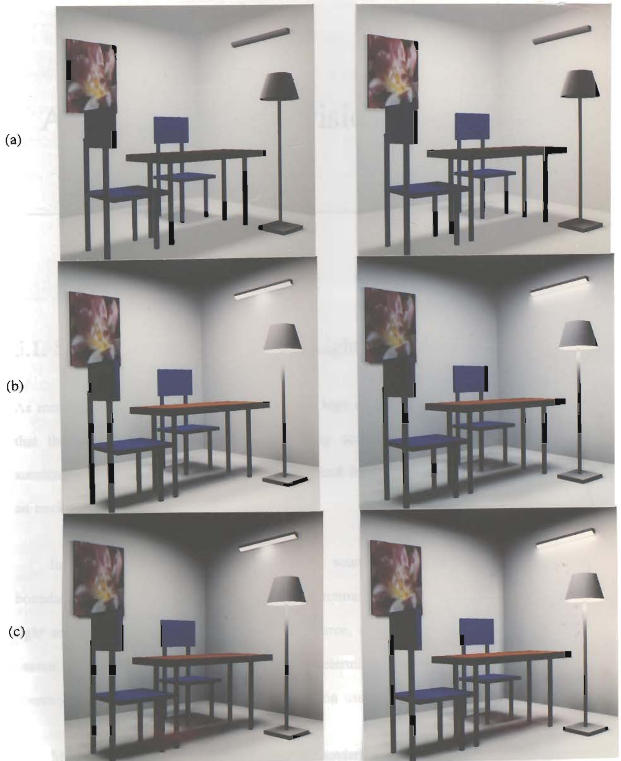
Figure 4.5. A room after the light of (a) 1 source (totally 9 subsources) is shot; (b) 2 sources (totally 18 subsources) are shot; (c) 5 sources (totally 33 subsources) are shot.
